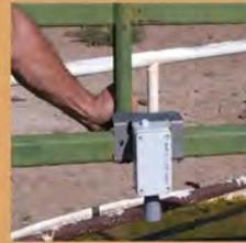
LoRa-enabled DecentLab™ real-time water level sensor
